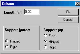
The length and the upper and lower end-support are stated for columns.
